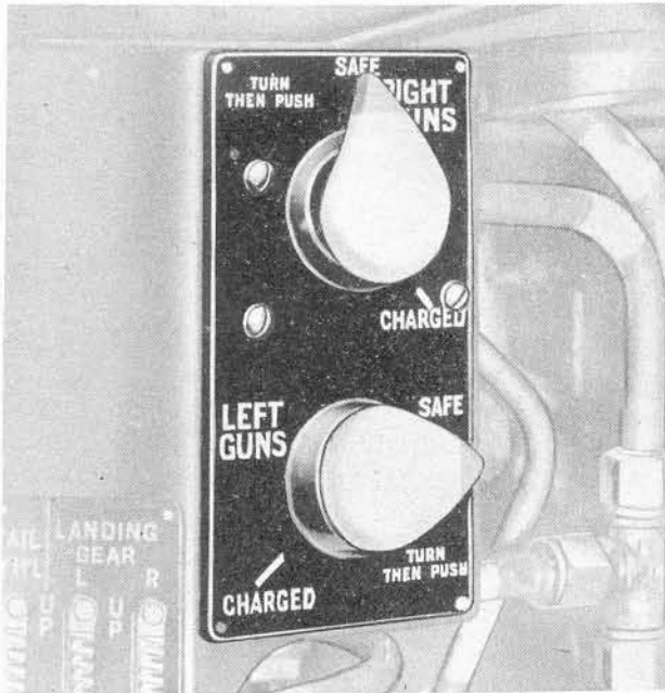
Figure 16—Gun Charging Controls
