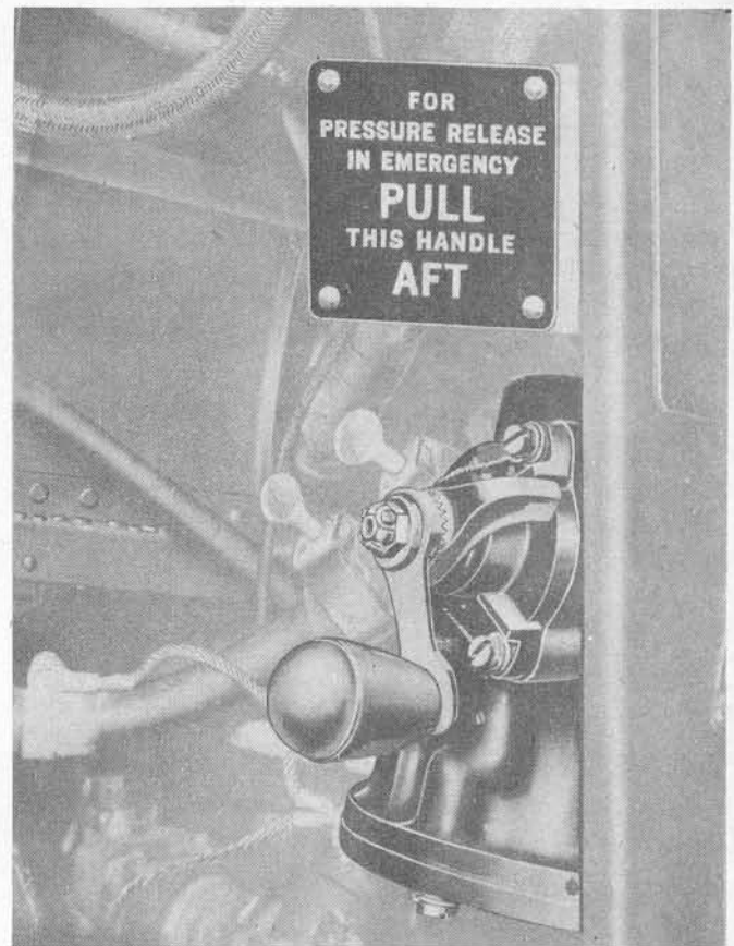
Figure 25—Main Fuel Tank Pressure Regulator
