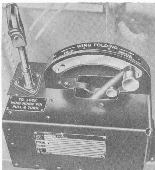
Figure 14—Wing Folding and Locking Controls
